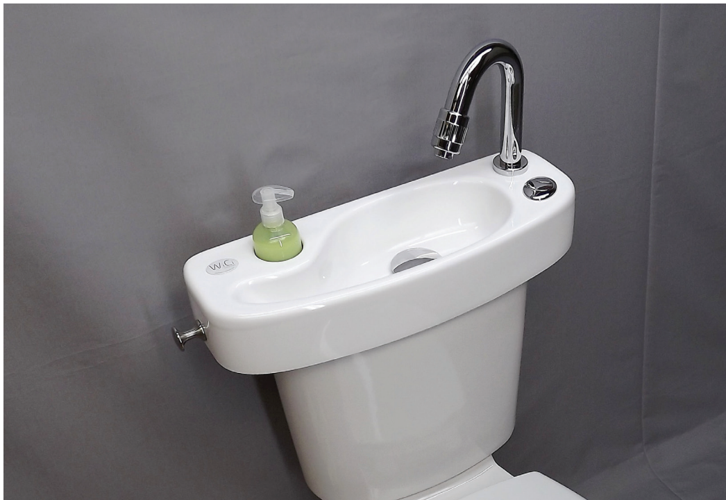
Photo 15: WiCi: the water you use to wash your hands will be used by next person to flush the toilet, and so on.
